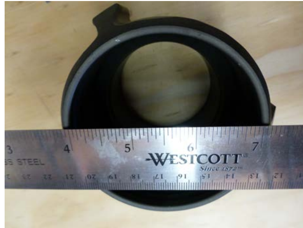
Figure A 3-inch Coupling Bowl for 2.5-inch DJ Nylon Rubber lined hose
