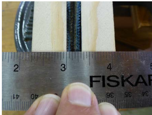
Figure D 0.3125-inch DJ Nylon & Rubber Liner Material Thickness in 2.5-inch Hose
