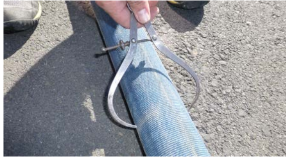
Figure E External caliper measurement of diameter of charged 2.5inch hose
