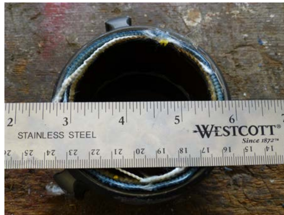
Figure B 2.5-inch hose cut off at the coupling
