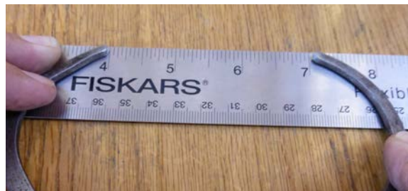
Figure F External caliper measurement of diameter of 2.5-inch hose
