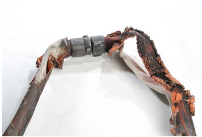
Image #1 Fire damaged traditionally constructed rubber lined, nylon double jacketed hose
