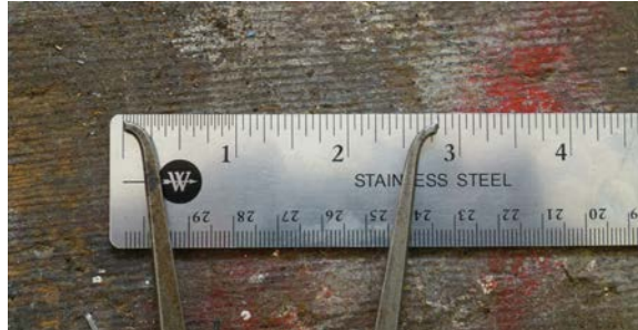
Figure# C 2.8125-inches Expansion Ring Measurement in 2.5-inch Nylon DJ Rubber Lined hose
